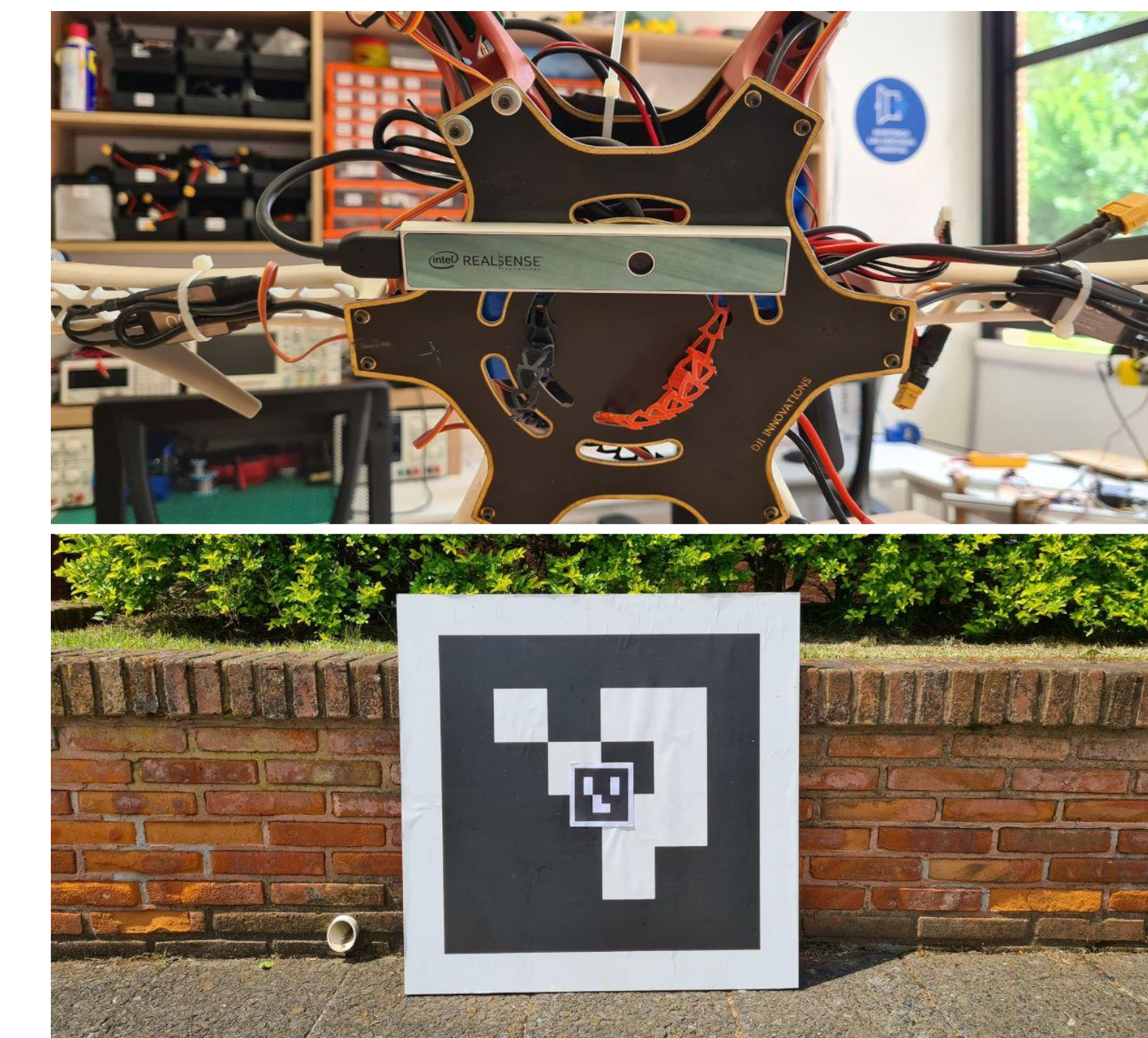
Fig. 5: Intel® RealSense™ mounted in hexarotor and fiducial marker.
